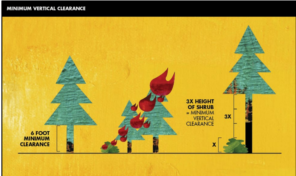
Figure J.4. Minimum vertical clearance.
